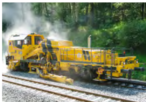
Fig. 5-28: Ballast distributing and profiling machines: R21 (MATISA, left) and USP2010SWS (Plasser & Theurer, right)
